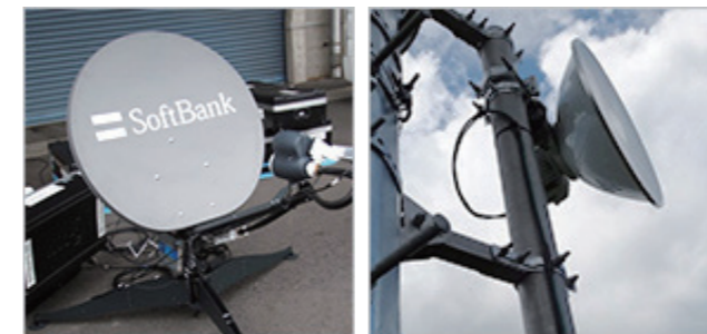
Mobile satellite antennas Microwave relays
