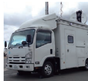
Mobile base station vehicles
