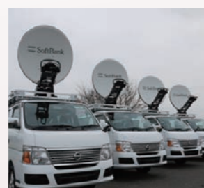
Portable Mobile Base Stations
