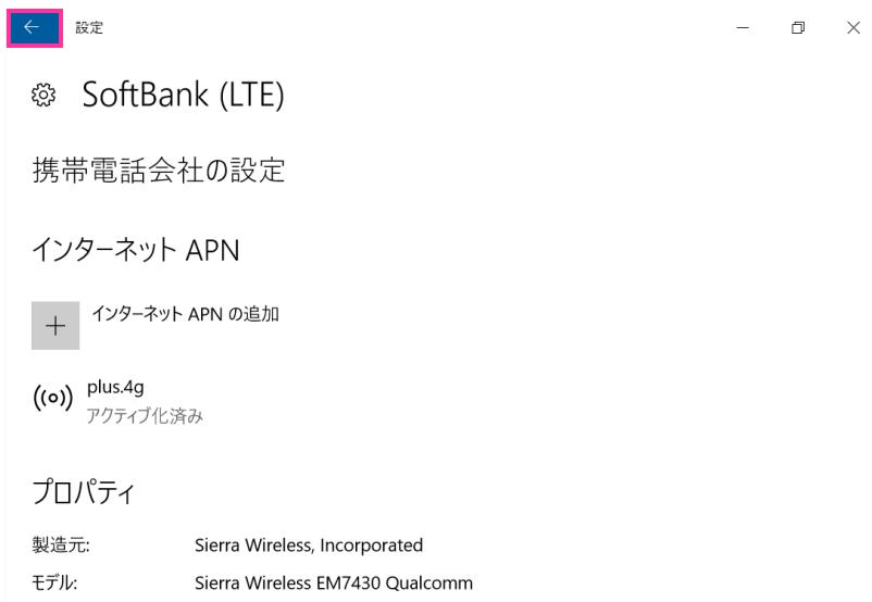
The SoftBank (LTE) APN configuration screen is shown. The APN 'plus.4g' is listed with the status 'アクティベ化済み' (Activated).
