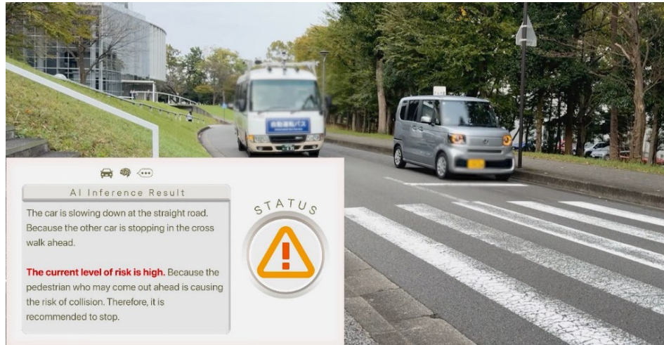
Figure 18. Inference results of multimodal AI when a vehicle is stopped in front of a crosswalk
