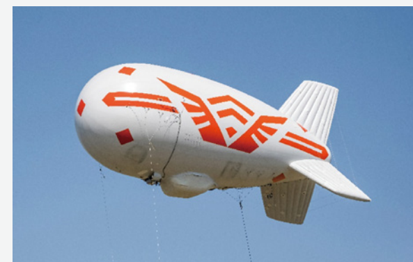
Altaeros's high-altitude tethered aerostat used in the field trial in Hokkaido
