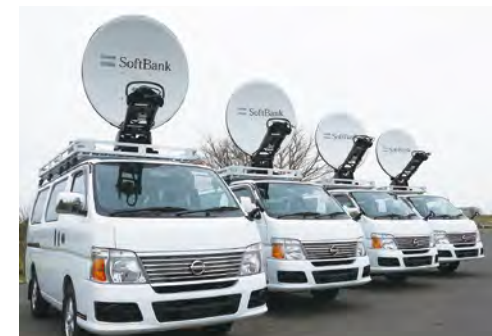
Portable mobile base stations
