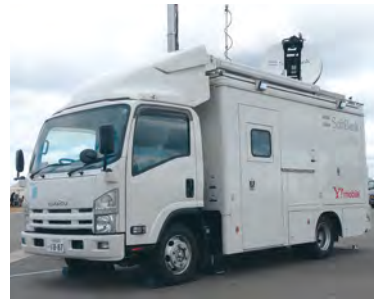
Mobile Base Station Vehicle
