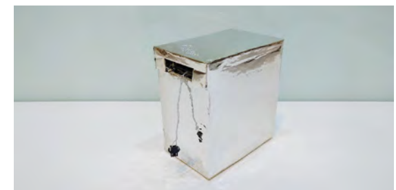
Battery pack for HAPS
