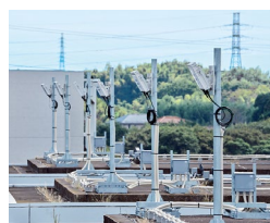
Base station clusters arranged in high density to simulate an urban area
