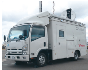
Mobile Base Station Vehicle
